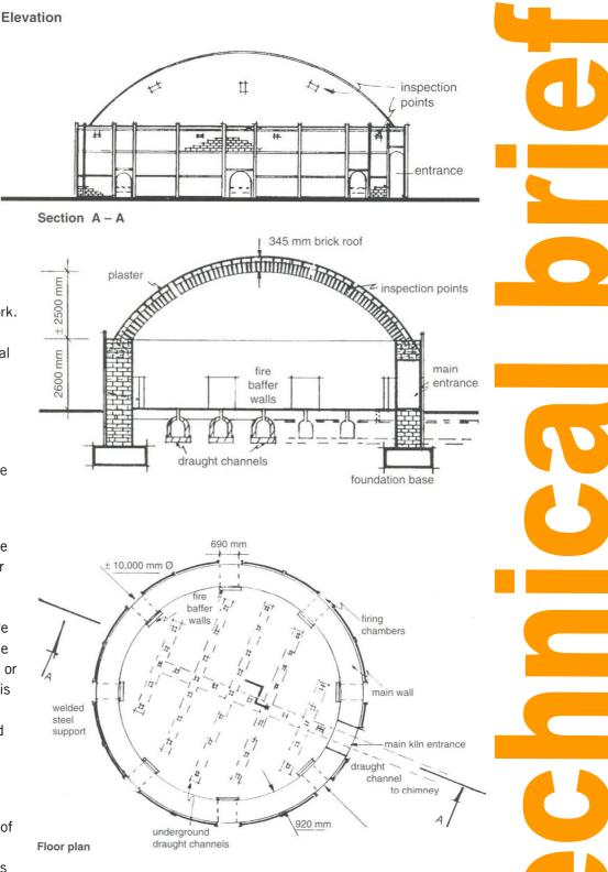
Figure 2: Plan, section and elevation of an igloo kiln
